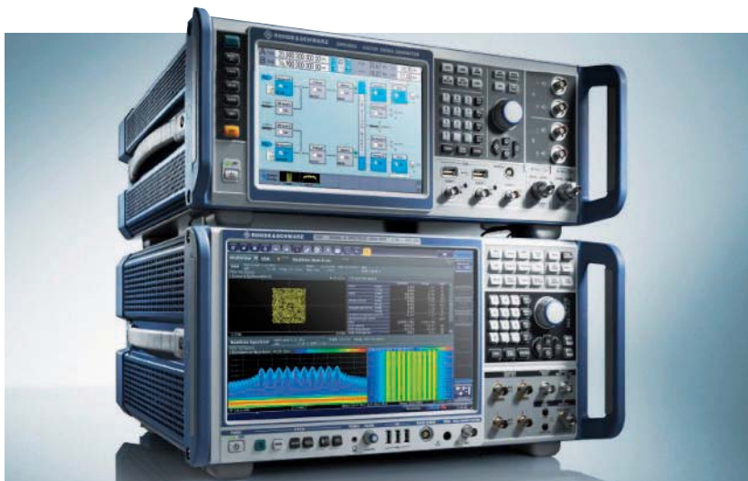
1. The two instruments at the heart of the radar target generator system are the R&S FSW signal and spectrum analyzer (bottom) and the R&S SMW200A vector signal generator (top).
