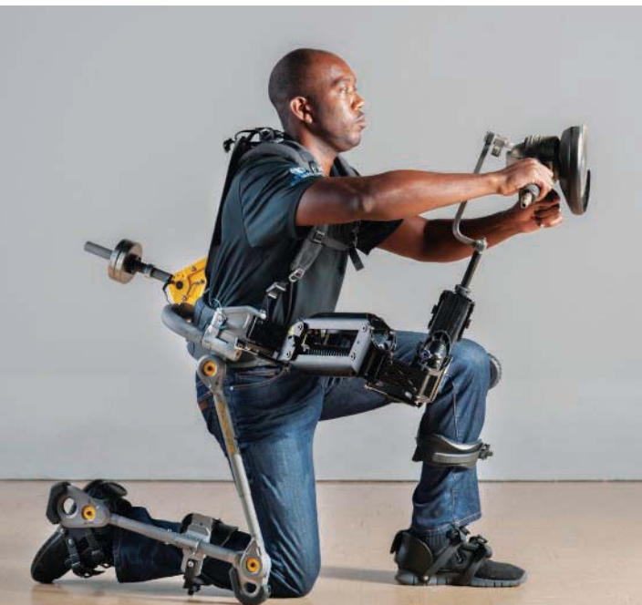
FORTIS is capable of holding objects up to 36 pounds.
