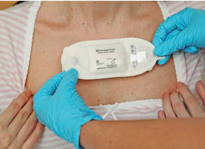
Sensium Healthcare Sensium Vitalis sensor is a patch that provides patient status including heart-rate, respiration, and local temperature.
