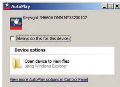
1. An AutoPlay dialog box such as this appears when connecting a PC to an instrument with USB.
