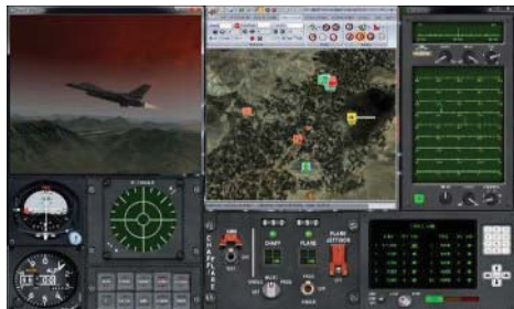
2. EW simulators in the EWSIM product line employ physics-based models to recreate aerodynamic models. [Screenshot courtesy of Electronic Warfare Simulation Corp. ( www.ewsim.com )]
